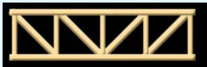
Pratt truss for bridges
