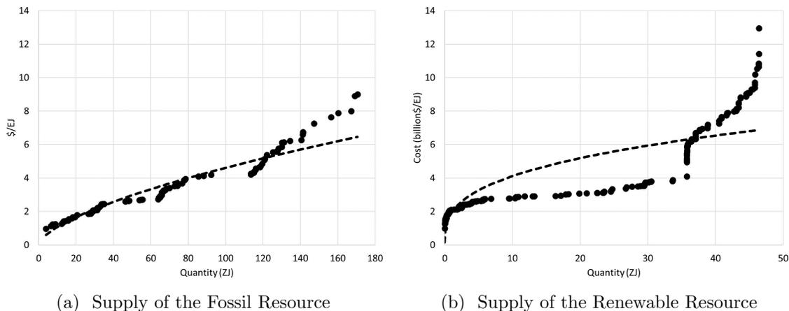
Figure 6: The constructed supply curves (solid points) for the fossil resource (left) and the renewable resource (right), as well as the fitted curves (dashed lines) used in the simulations. Note that the scale of the horizontal axis differs between the panels.
