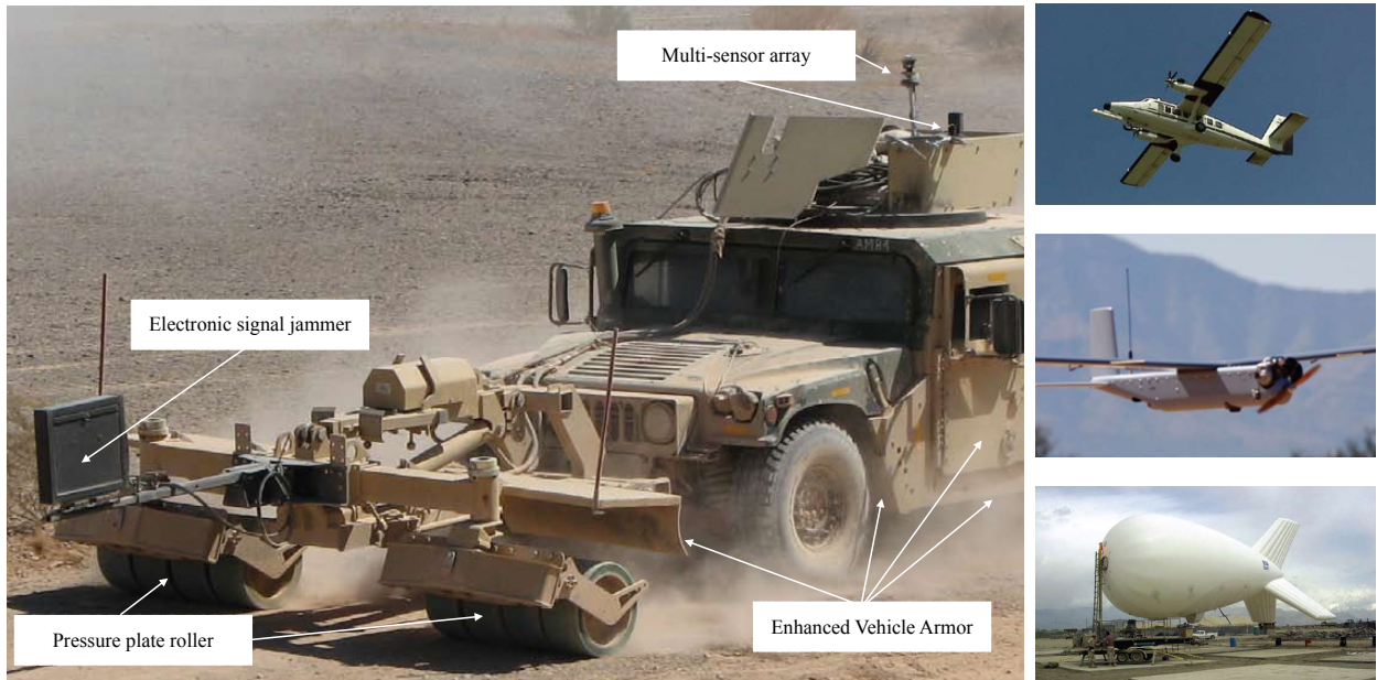
(a) IED Thwart devices on Humvee
