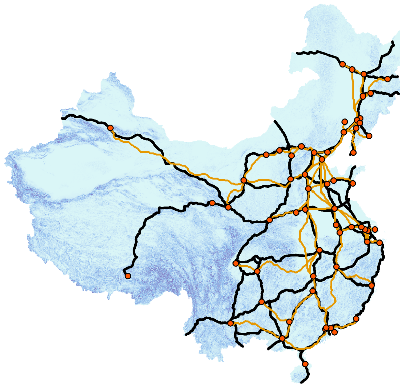
The map shows the approximation of the optimal highway network in China based on the heuristic algorithm without the constraint that all targeted cities are connected. The background shows the slope of the terrain of mainland China. The nodes show the location of all cities with a population of at least 500,000 and all provincial capitals.
