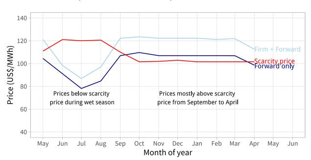
**Figure 9:** Comparison of monthly mean prices between counterfactual scenarios for the low water case (10% below 2015 water levels)
